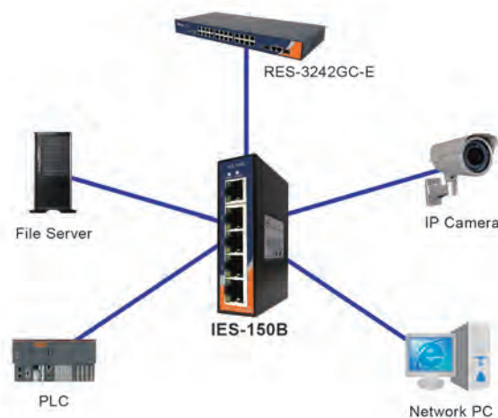
Connections of Ethernet devices
