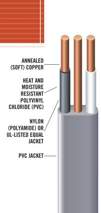
Underground Feeder and Branch Circuit Cable
